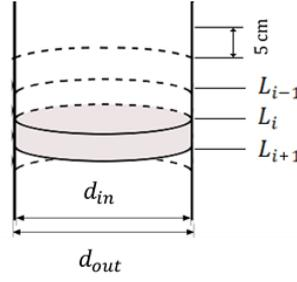
Figure 1. Discretization scheme of the calciner model.
