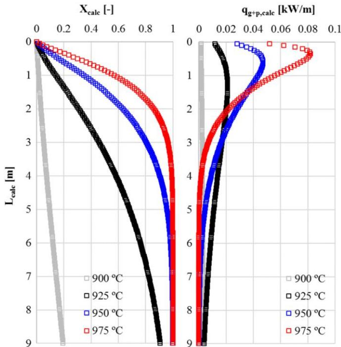
Figure 2. (a) Conversion profiles of the calciner ( $X$ ) vs. length, (b) required heat per unit length ( $q$ ) vs. length.
