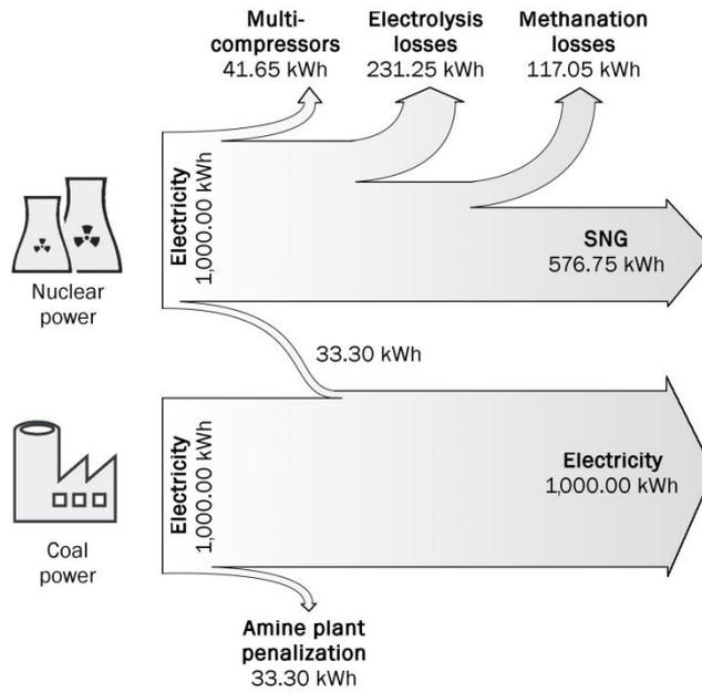
Figure 4. Sankey diagram of the displacement of electricity through Power to Gas.
