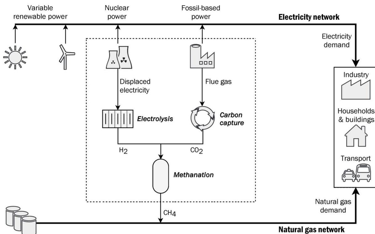
Figure 1. Schematic diagram of the nuclear power displacement through Power to Gas
