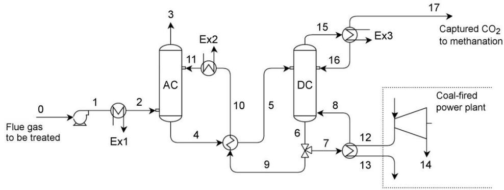
Figure 2. Scheme of the amine carbon capture plant
