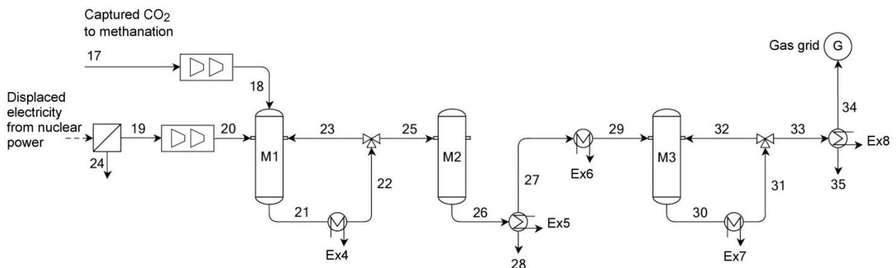
Figure 3. Scheme of the Power to Gas plant
