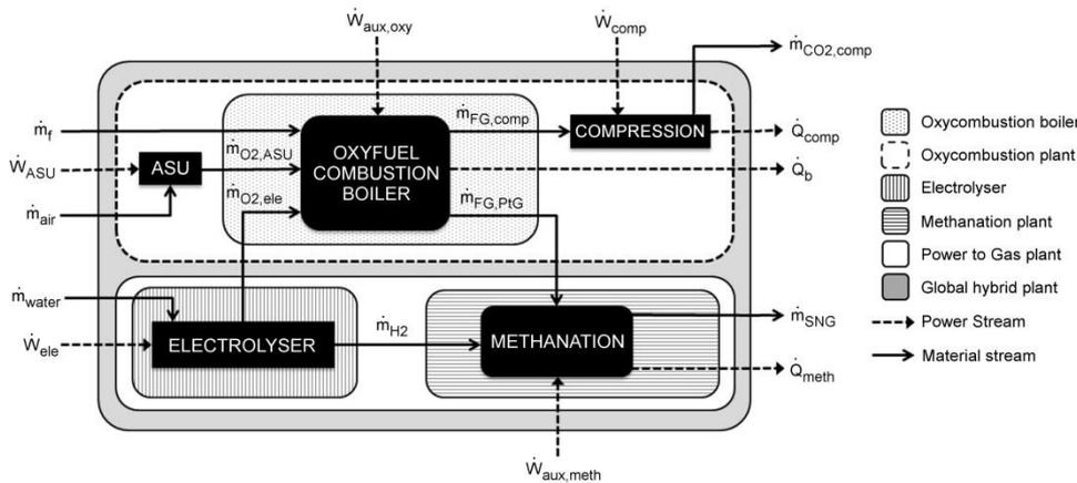
**Figure 1.** Scheme of the hybrid Power to Gas-Biomass oxyfuel boiler system.
