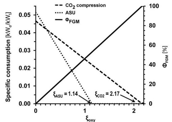
**Figure 2.** Specific consumptions [kW<sub>e</sub>/kW<sub>t</sub>] and methanised flue gas [%] vs  $\xi_{oxy}$
